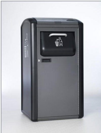
Figure 5: A solar panel on top of the BigBelly bins power a trash compactor inside the bin, and a wireless sensor alerts collection agencies when the bin is full. (Source: BigBelly Solar)
